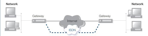
Exchange of the dynamic IP-addresses via ISDN
